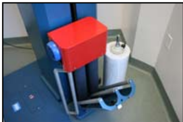
Easily accessible guide rollers for quick and easy changeover.
