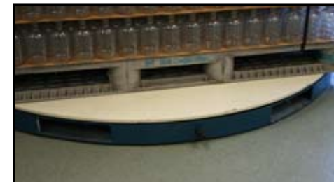
Easy forklift relocation with inserts on the front of the machine.
