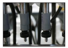
**AccuVac** fillers deliver free flowing liquid product into a rigid container until the fill level reaches a specific fill mark even if there are slight variations in the size or shapes of bottles and jars. It is
