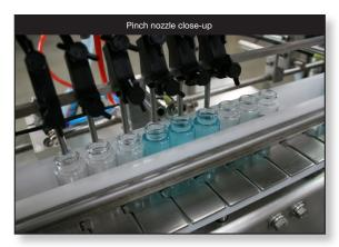
The **Auto Pinch Series Fillers** are automatic timed flow volumetric filling machines capable of filling water thin liquids to light oils and creams at speeds of up to 100 containers per minute. Minimal contact parts (hose and pump) make the **Auto Pinch Series** ideal for sanitary filling of food, pharmaceutical, cosmetic, and specialty products. The speed and ease of use make the **Auto Pinch** filler the perfect machines for medium speed small container filling operations.
