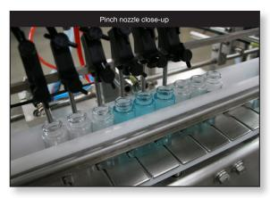
The **Pinch Series Fillers** are timed flow volumetric fillers designed to fill water thin liquids to oils and creams. All the contact parts can be easily cleaned and are autoclavable which makes the machine ideal for the medical, pharmaceutical, food, cosmetic, and specialty industries.
