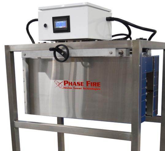
The G3 Shrink Tunnels utilize the same infrared quartz convection heat and insulated recirculating system as the G1 Series Tunnels. However the G3 Shrink Tunnels have the added benefit of an adjustable width allowing them to accommodate a larger variety of container sizes.
