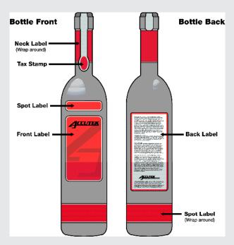
A single RL Series Rotary Labeler can have multiple label heads equipped allowing them to place several different labels onto one container all within a single system. Label placement can be on the front, back, neck, or any arrangement of locations. Wrap around labels can also be applied in combination with spot labels. The Biner Ellison RL Series Labelers are also capable of applying a Tax Stamp onto containers.
