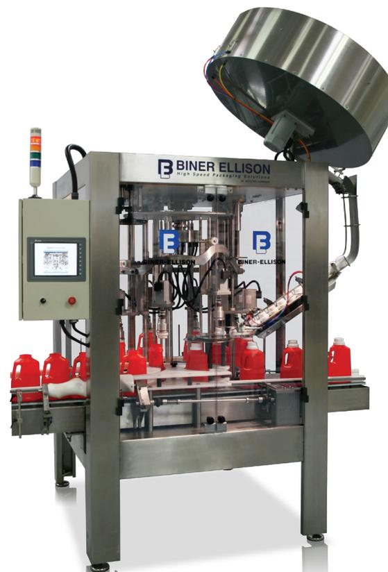
The **Biner Ellison RC Series Cappers** are versatile rotary capping systems design to complement high speed rotary bottling equipment. These flexible rotary cappers continuously sort, apply, and torque caps to a variety of different container sizes and shapes.
