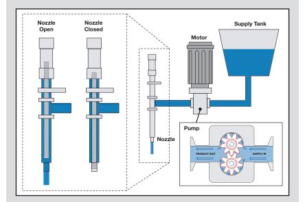
PD fillers measure and deliver the product into the container by utilizing a PD pump head. The standard types of pump heads used are Gear Pump Heads and Flexible Impeller Pump Heads. A Pneumatic Clutch couples the Drive Motor to the Pump Head. A high-speed counter provides feedback to the PLC by counting fractions of revolutions of the motor rotation.
