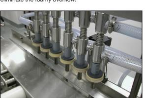
The APOF units are very easy to setup and maintain. Each machine includes a sanitary stainless steel manifold with a quick clean connection. A touch screen control system records job settings for fast and simple changeovers, setup instructions, and offers a trouble shooting help menu.
