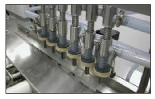
The APOF units are very easy to setup and maintain. Each machine includes a sanitary stainless steel manifold with a quick clean connection. A touch screen control system records job settings for fast and simple changeovers, setup instructions, and offers a trouble shooting help menu.
