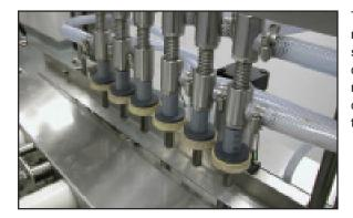
The APOF units are very easy to setup and maintain. Each machine includes a sanitary stainless steel manifold with a quick clean connection. A touch screen control system records job settings for fast and simple changeovers, setup instructions, and offers a trouble shooting help menu.
