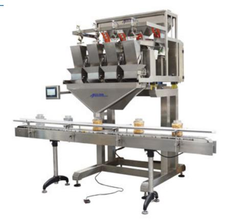
An automatic granular product weight filling machine that can be ordered with two filling channels that funnel into a single fill head, or four filling channels that funneled into two filling heads. Accutek vibratory feeders are the ideal solution for dry granular products that require precision weighing. The vibrating delivery channels that feed product to the load cells avoid damage normally encountered with feed screw or auger systems.
