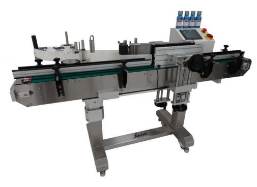
The labelers accommodate plastic, metal, fiber, and glass containers, offering versatility for diverse packaging needs. The APS-106-F Series Labeler provides a comprehensive automated labeling solution for various industries. Their capacity to manage diverse label sizes, materials, and high-speed operations, along with user-friendly software for quick adjustments, adds value to packaging lines seeking efficient and reliable labeling processes.
